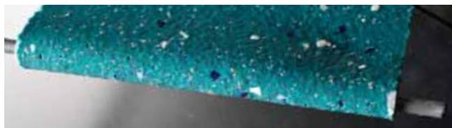
This picture shows Polysafe Astral PUR; shade 4220 Aquarius, tested around a 4mm mandrel. No whitening or cracking is observed. This test by far exceeds the requirements set in EN 13845 - the European Norm for Safety Flooring.
